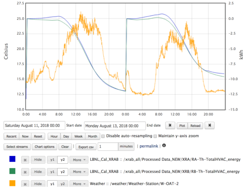
Figure 2. Calibration results – Cumulative thermal load comparison for each cell under identical conditions.
