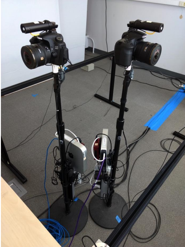
Figure 7. High-dynamic-range luminance mapping apparatus.
